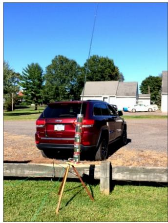
tests mounted on a tripod with only three 8 foot "radials", I received good signal reports from Cuba, Washington State and Wyoming on 15 Meter CW transmitting only 25 Watts. Local 10 Meter contacts were significantly better with the Coffee Can Vertical than the Mobile's HV7A. 73. **Griff NE3I**
